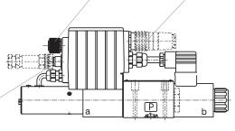
**K3** - Conektor M12x1 (5 PIN) External feedback signal (for configurations E03 and E04S01 only).
