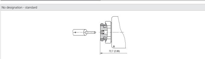
In case of solenoid malfunction or power failure, the spool of the valve can be shifted by manual override as long as the pressure in port T does not exceed 25 bar (363 PSI). For alternative manual overrides contact our technical support.
