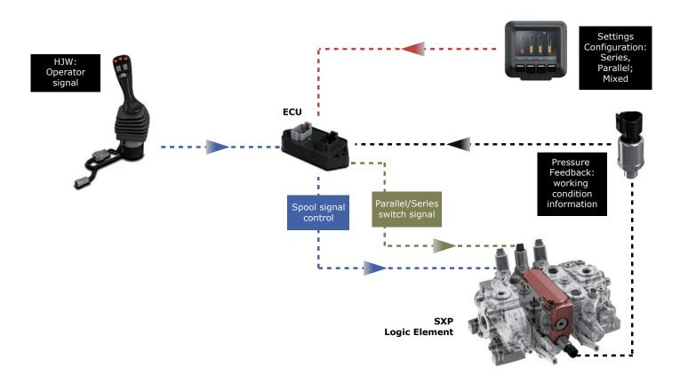
The work mode can be simply set by selecting it on the control panel.
