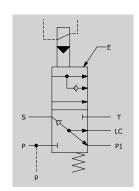
In this configuration the valve works as a typical **PARALLEL** circuit.
